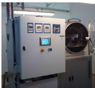
Fig. 1 The device to deposit thin metallic coatings onto various textile media
