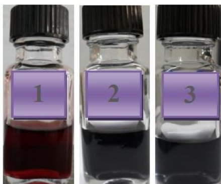
Figure 1. Samples of AuNPs stabilized by PVP with M_n = 10 \cdot 10^3 (1), 40 \cdot 10^3 (2) and 350 \cdot 10^3 (3)
