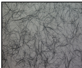
Figure 1. Conductive veil, fabricated from polyamide with 1% wt. of CNTs.
