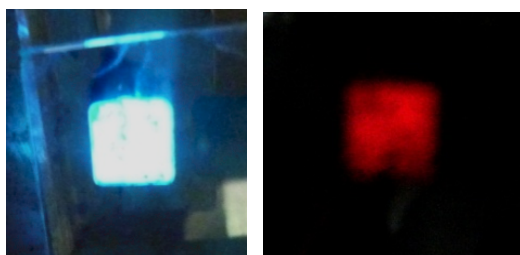
Figure 1. Photograph of an OLED using a blend of the photosensitive polymer and polyfluorene as emitting layer before (left) and after (right) the photochemical immobilization of the Ru(II) complex.
