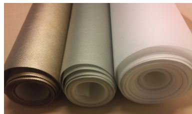
Fig. 2 Barrier materials with different metal alloy coatings - examples
