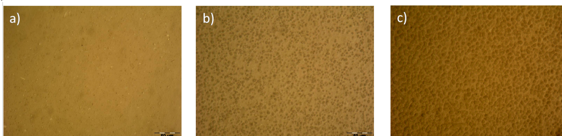
Figure 3. Optical micrographs of foamed ink layers a) prior to and b,c) after UV illumination
