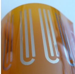
Figure 1. inkjet printed platinum electrodes on flexible polymer substrate (Kapton®) for use as biosensors.
