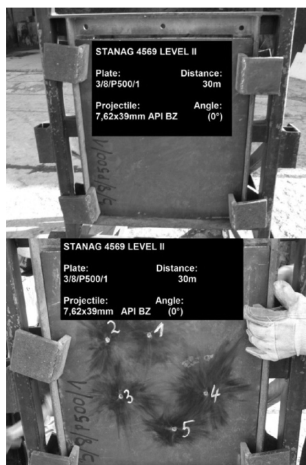
Fig. 16. Test plate before and after the ballistic test
