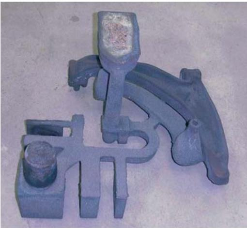
**Figure 18.** Cluster with test castings
