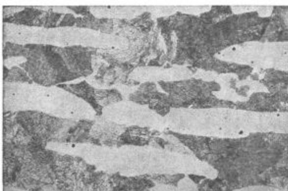
Slika 3 Struktura jekla 2 v normaliziranem stanju (500 ×) Fig. 3 Structure of steel 2 as normalized (500 ×)
