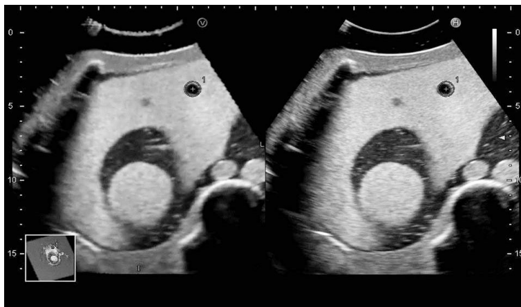
FIGURE 1. RVS synchronization using 3DUS data from a phantom model. US-MPR images from the 3D data (left) and real-time US images (right) are synchronized on the same US monitor. Furthermore, synchronized spherical markers (+, the center of the spherical marker) are displayed along the contour of a spherical structure of the phantom model on synchronized US-MPR and real-time US images.
