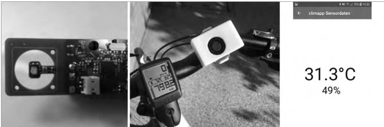
Figure 4: Prototype of the climapp sensor, which collects mobile data on local climate conditions (source: authors).
