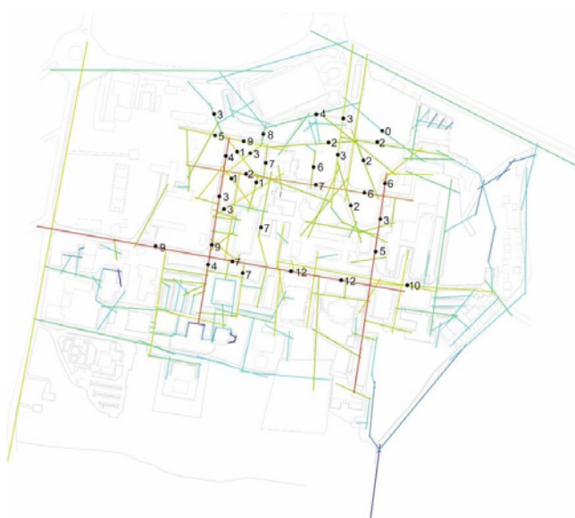
Figure 9: Average number of people per gate plotted against Global Integration RN map. University Clinical Centre of Kosovo.
