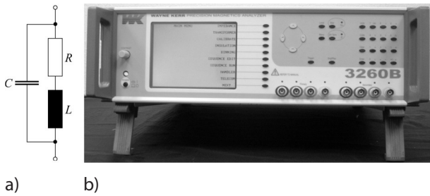
Figure 9: High frequency equivalent circuit model (a) of the inductor, Wayne-Kerr 3260-B impedance analyzer (b) used for measurements.
