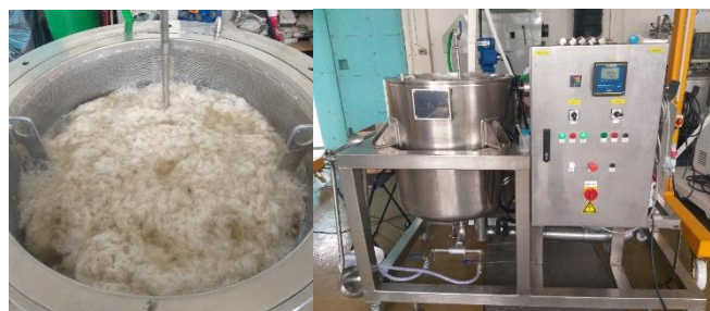
Figure: Enzymatic hydrolysis of cellulose textile waste material (left) and pilot-scale batch reactor for cellulose material degradation (right)
