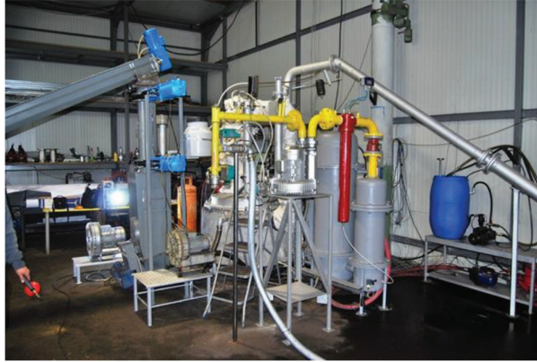
Figure 6: Prototype gasifier with 600 kW th input power
