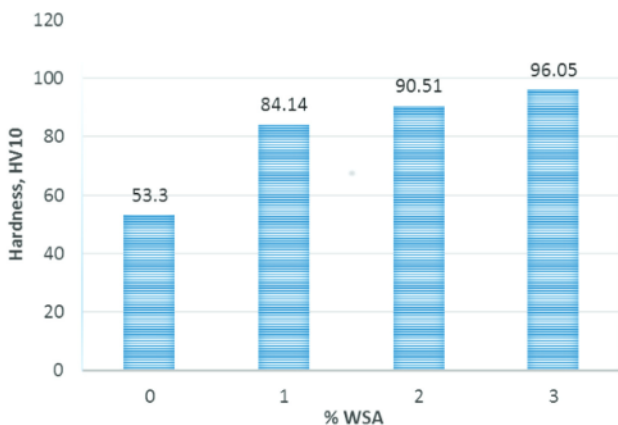
Figure 6: Variation in the hardness with the weight fraction of WSA
