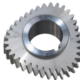
Fig. 7. 3 rd order elliptic helical gear, hobbled
