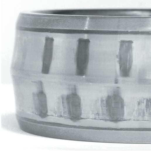
Fig. 10. Damaged bearing of lever pivot
