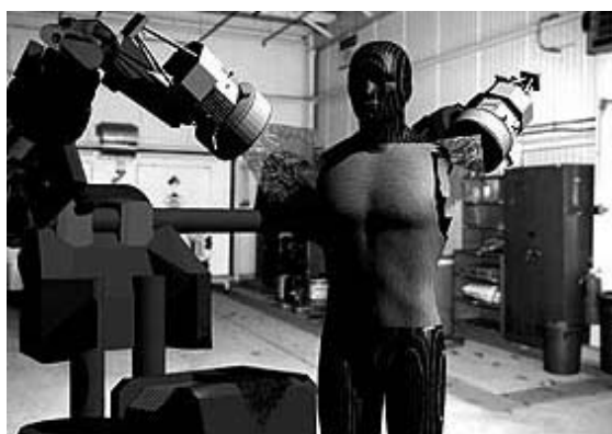
Figure 3: Direct depositing of nanofibres on the surface of a garment with an electrospinning process
