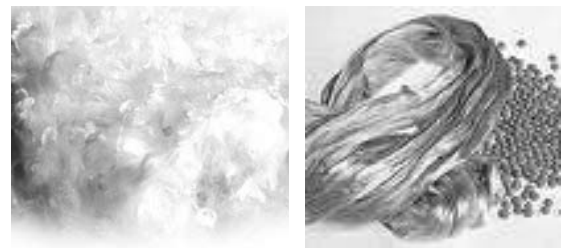
Figure 21: Soyabean protein fibres – raw (left) and bleached (right)
