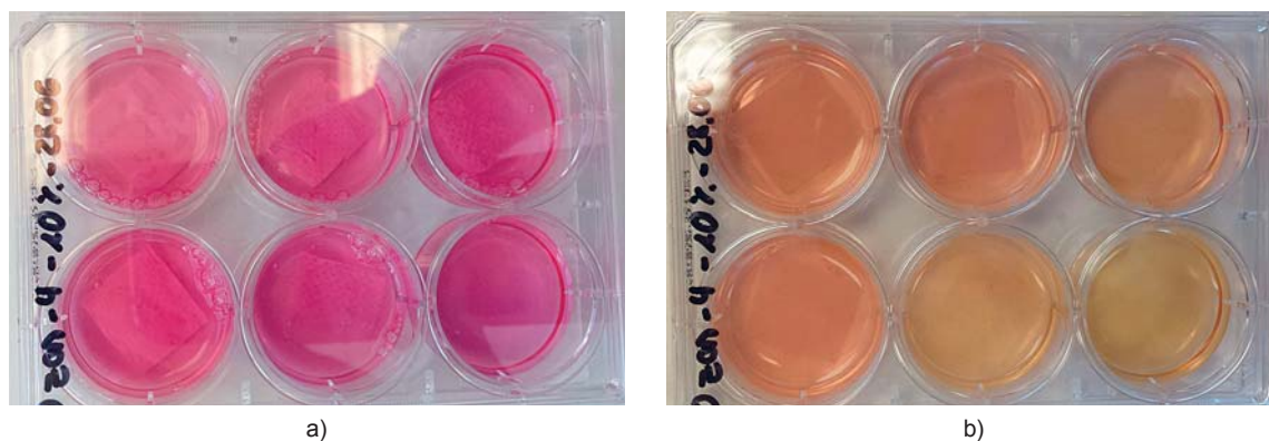
Figure 4: 6-well plate with ozone-sterilized nanofibrous mats (10% gelatine) in culture medium (only medium in lower right well as reference) with CHO DP-12 cells, (a) start of cultivation, (b) end of cultivation at day 5
