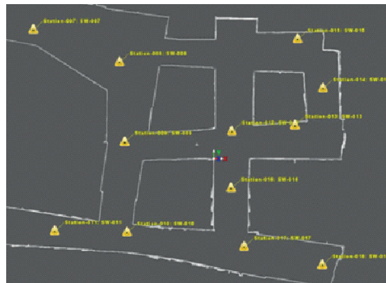
Figure 1: Photo from the field work - 3D terrestrial laser scanner (left), a scheme of scan positions inside the quarry (right).
