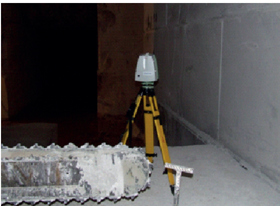
Figure 1: Photo from the field work - 3D terrestrial laser scanner (left), a scheme of scan positions inside the quarry (right).
