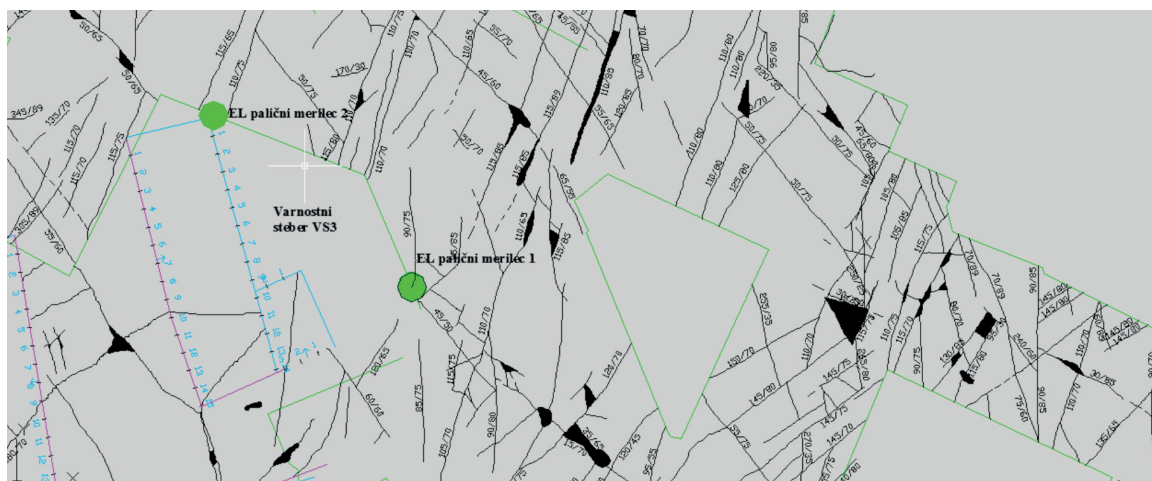
Figure 4: Map of the rock discontinuity orientations and locations (green circle) of EL beams gauges installations in quarry Lipica II [11] .
