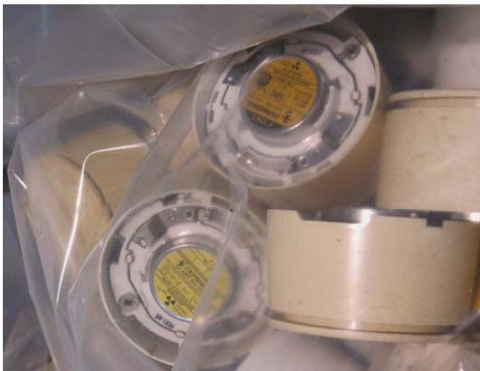
Figure 17: Disused ionizing smoke detectors
