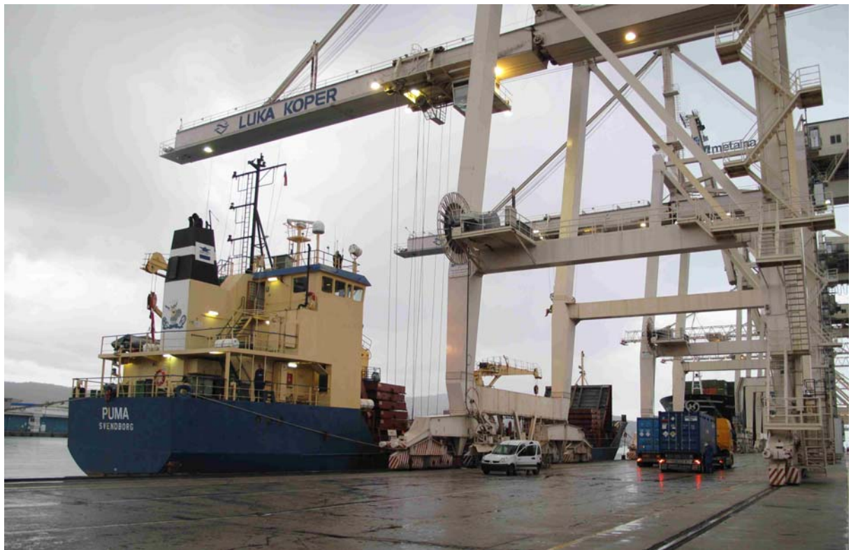
Figure 16: Loading of containers with transfer casks on a specially equipped vessel in the Port of Koper
