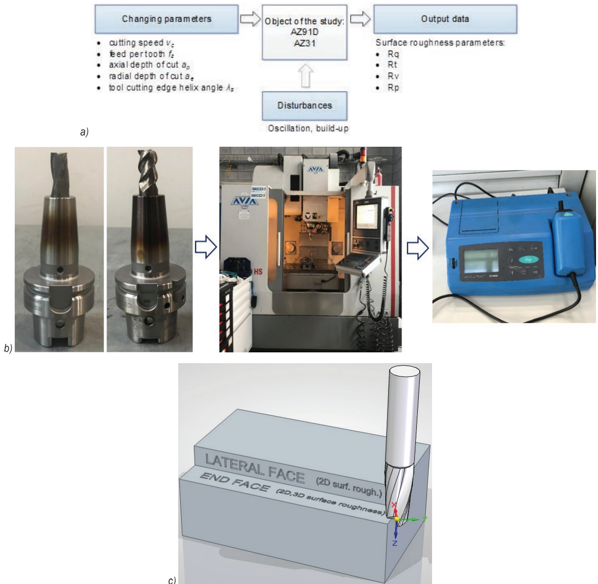
Fig. 1. Research scheme: a) the test set-up, b) the measurement equipment (end mill, milling machine and 2D profilographometer), and c) milling visualization with the roughness measurement model with end face and lateral face on the workpiece surfaces
