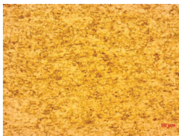
Fig. 6. Investigation of a) the microstructure, and b) chemical compositions of Ti6Al4V; produced by EDX results
