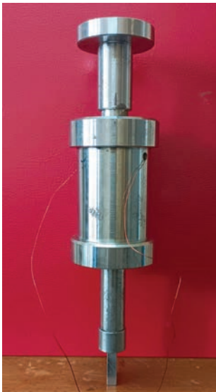
Fig. 2. The prototype of a dual-acting MRE damper
