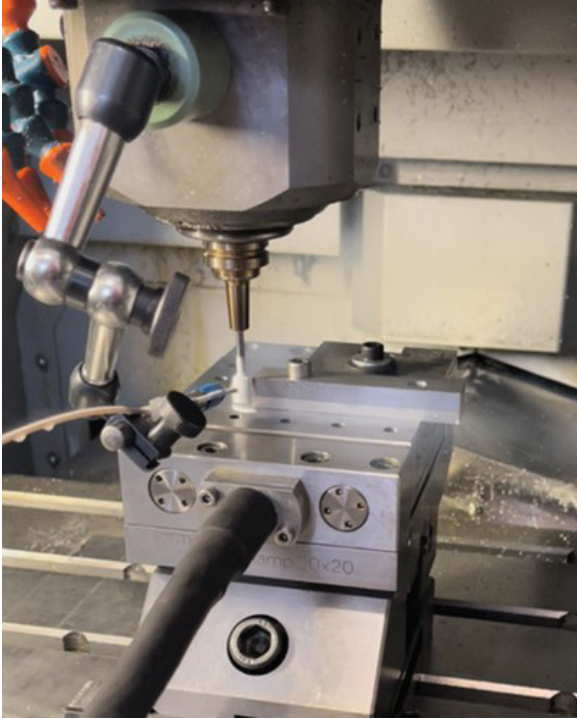
Fig. 3. LCO 2 -MQL grinding set up
