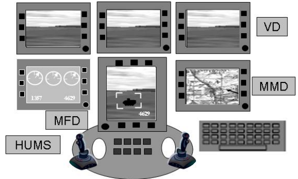
Fig. 3. AFV crew station block diagram
