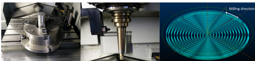
Fig. 2 Workpiece clamping (left), shrink-fit ceramic tool clamping (middle), spiral milling strategy (right) [13]
