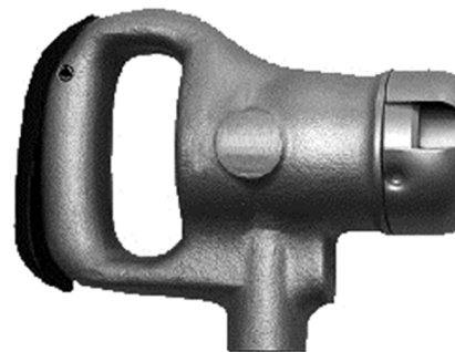
Fig. 6. Existing pneumatic hammer (handle)
