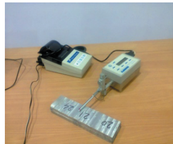
Fig. 2. Surface roughness measurement using Surtronic 3+
