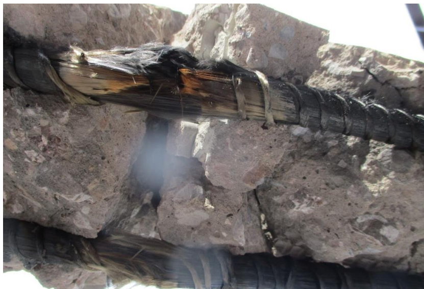
Fig. 7. HFRP Bars After the Matrix Evaporated in Specimen Reinforced with 14 mm HFRP Bars
