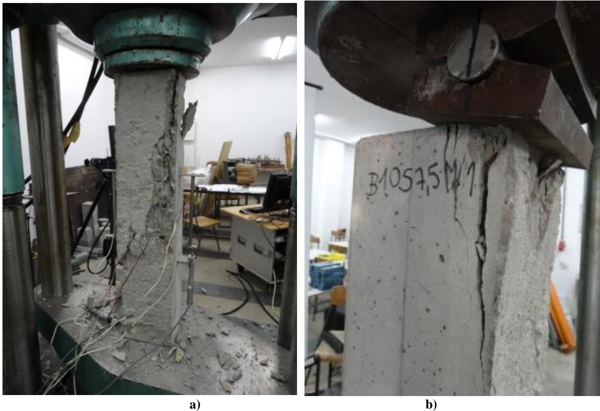
Fig. 8. Destruction mechanisms (a) axially loaded members (with HFRP reinforcement) (b) members loaded with eccentric force (with BFRP reinforcement).
