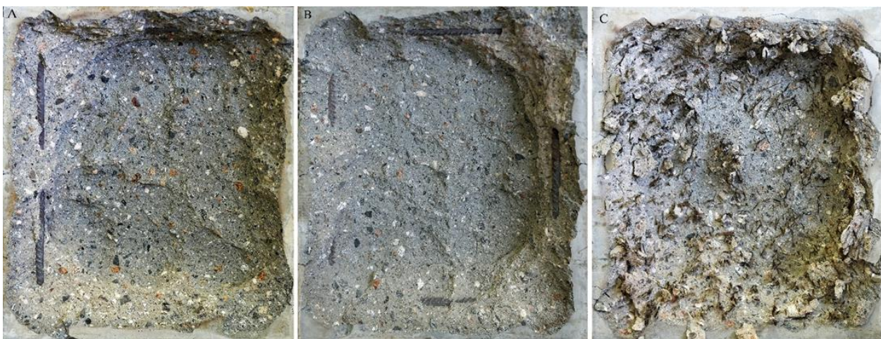
Figure 7 – Test specimens after fire testing. Left = reference concrete. Centre = concrete with 0.5 % fibres of type C. Right = concrete with 0.5 % fibres of type M. Photo: A M Mohaghegh.
