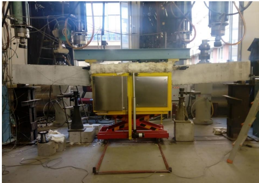
Fig. 6. Test Setup of Specimen, Beam Reinforced With 14 mm Two BFRP Bars, Being Heated and Loaded
