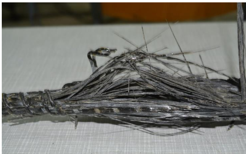
Fig. 4. Destruction of 8 mm diameter HFRP bar.
