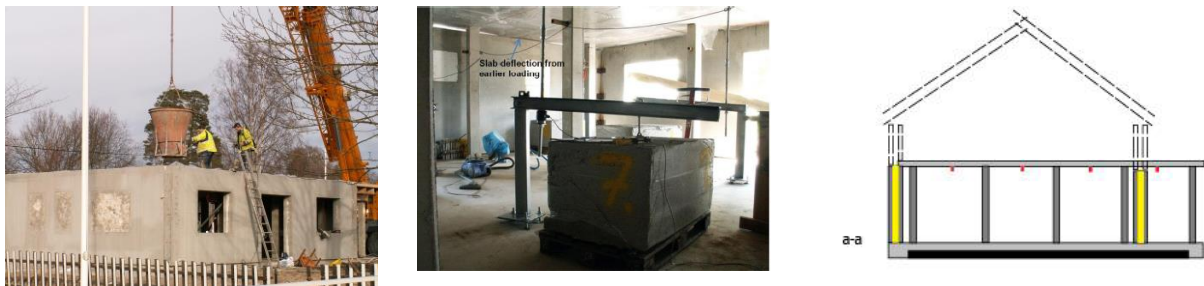
Figure 1. Full-scale tests on elevated fibre concrete slab on columns. From Hedebratt (2012).
