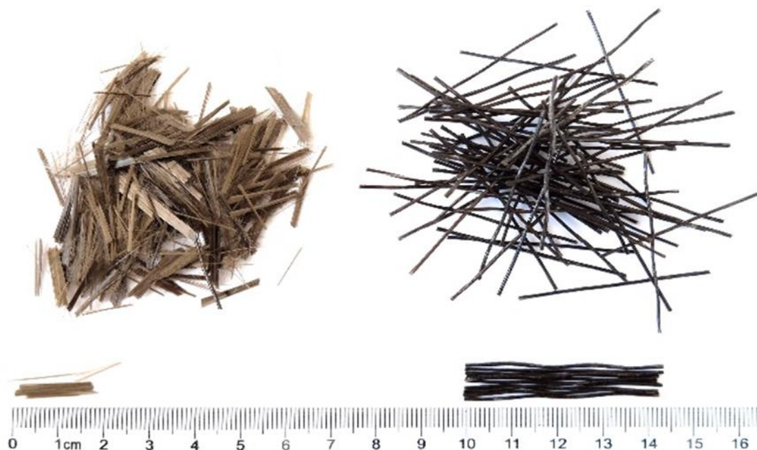
Figure 5 – Two types of basalt fibres. To the left chopped fibres (here denoted type C). To the right, bar-shaped fibres (often called Minibars, here denoted type M). Photo: A M Mohaghegh.
