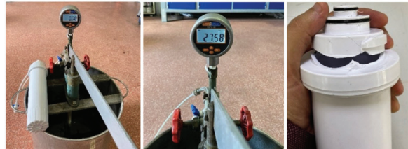
Fig. 9. Static test kit and the maximum pressure strength of 14/1 numbered test
