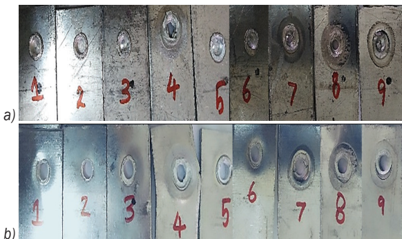
Fig. 6. Welded specimen a) Al 6061 top view, and b) AL 5058 bottom view
