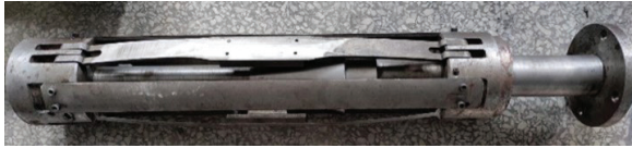
Fig. 20. Spring-type of anchoring mechanism
