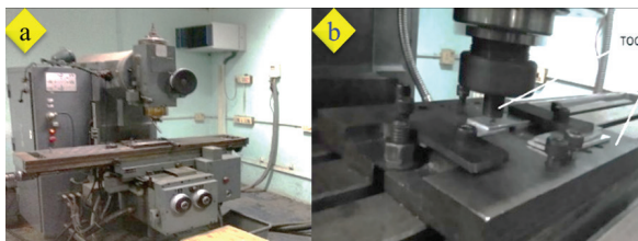
Fig. 1. a) Semi-automated vertical milling machine, b) specimen fixture
