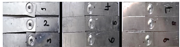
Fig. 4. Tensile test welded specimens
