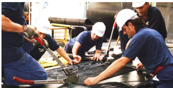
Fig. 2. Preparation process of a steel cord splice [RI-Belt Sud S.R.L.]
