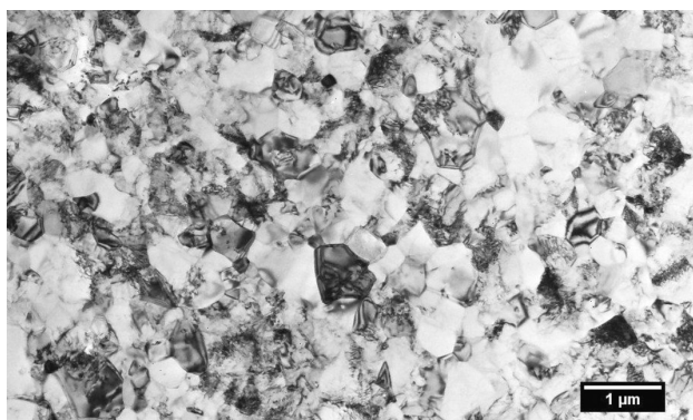
Figure 5: General view of Ti wire substructure after third pass at 200 °C
