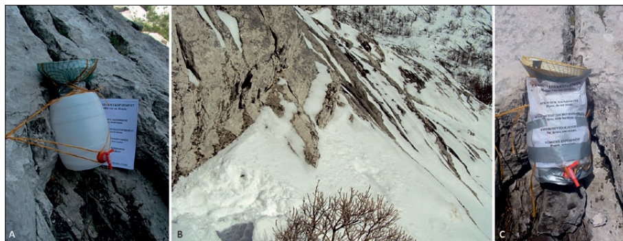
Fig. 4: Water collector in front of Spilja u Zubu Buljme Cave at 1250 m a.s.l.: a) after installing; b) under the snowdrift; c) damaged and repaired in situ (Photo: M. Surić and N. Lončar).
