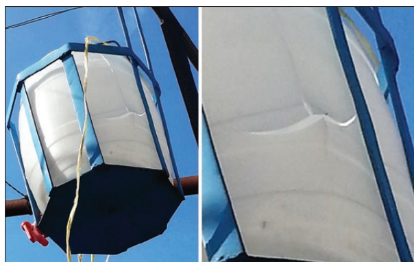
Fig. 5: Breakage of plastic water collector due to the long-term exposure to the direct sunlight (Photo: M. Surić).
