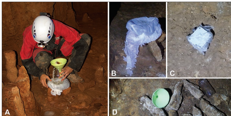
Fig. 10: Water collector and drip logger at the place of sampled MOD 32 stalagmite in Modrič Cave: a) initial installing and dismantled equipment b) bitten sand-filled plastic bag, c) displaced drip-logger and d) funnel (Photo: M. Surić).
