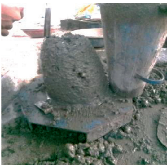
Figure 2: Workability of the concrete-slump test
