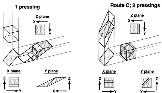
**Figure 3:** ECAP schema, shear plane passes through the channel, route C, first and second pressings<sup>6</sup>
