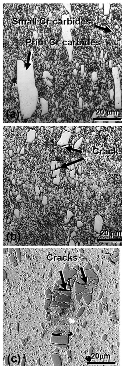
**Figure 8:** Microstructure of X210Cr12 steel: a) in the longitudinal section, b) in the annealed state and c) the state after ECAP
