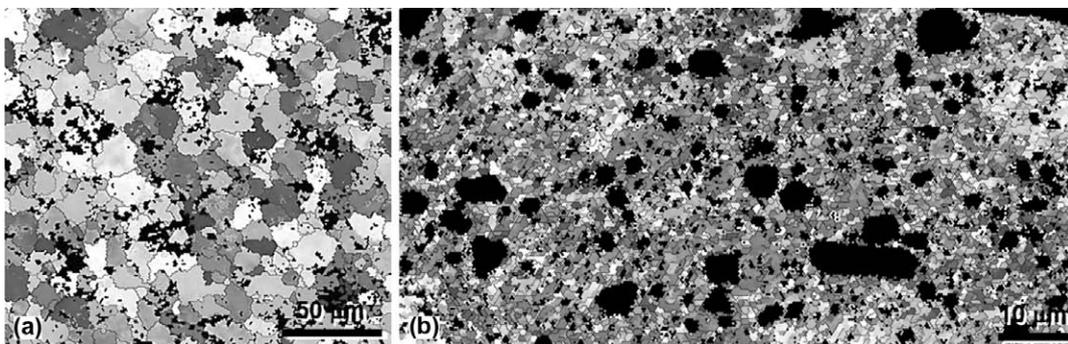
**Figure 5:** EBSD analysis of: a) the annealed state and b) modified state after ECAP
