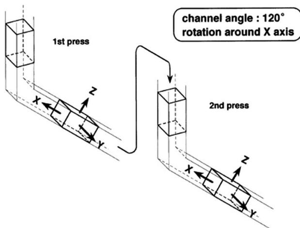
**Figure 2:** Channel with the bending angle of  $\Phi = 120^\circ$ <sup>5</sup>
