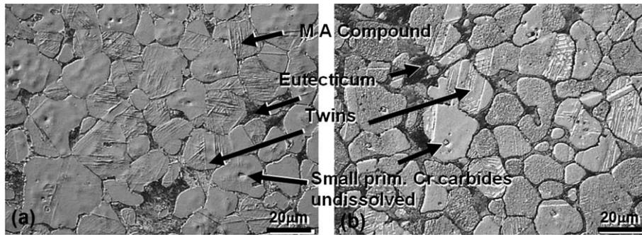
**Figure 9:** Structure after processing in the semi-solid state by mini-thixoforming: a) state of the annealed blank and b) state after ECAP; LM, polarized light, V<sub>2</sub>A etched
