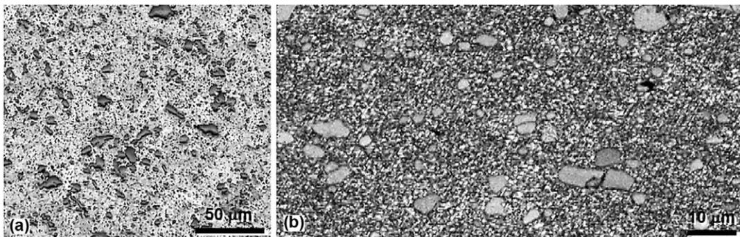
**Figure 6:** a) Band contrast of the annealed state and b) modified state after ECAP
