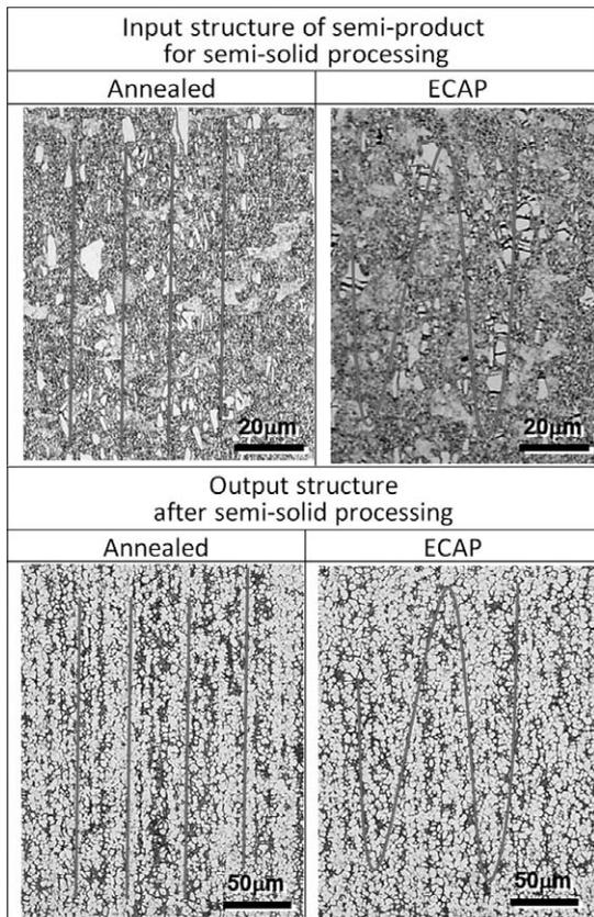
**Figure 10:** Characteristic arrangement of primary carbides and the eutectic network in the states before and after ECAP and semi-solid processing
