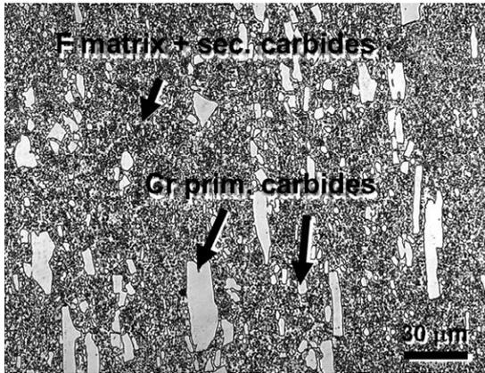
**Figure 1:** X210Cr12 steel microstructure in the soft-annealed state
