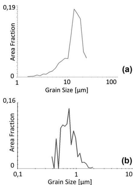
**Figure 7:** Results of the EBSD analysis: a) an evaluation of the grain size of the annealed state and b) the state after refinement using the ECAP process
