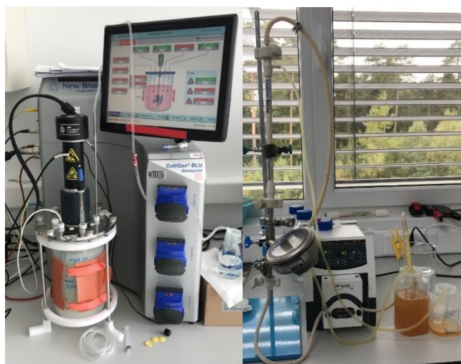
Figure 1: Glass bioreactor vessel with pH adjustment during fermentation (left) and laboratory filtration system for micro and ultrafiltration (right).
