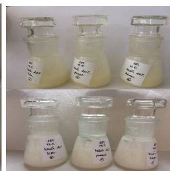
Figure 2. Yellowing of hydrogels (upper row) during stability study comparing to hydrogels at the beginning (lower row).
