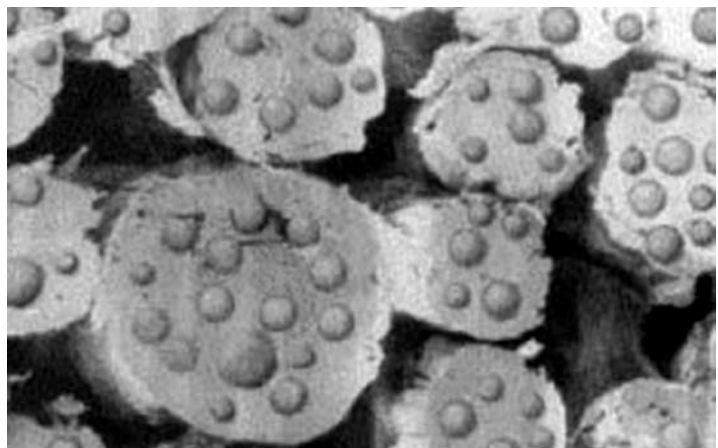
Figure 7: Incorporation of microcapsules into fibres (Outlast®) [15]
