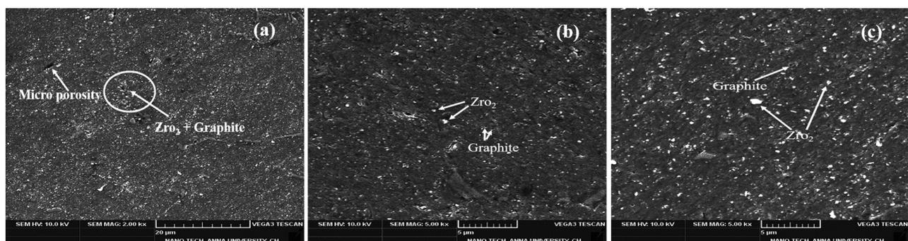
**Figure 1:** SEM images of fabricated composites: a) AHC5, b) AHC10, c) AHC15
