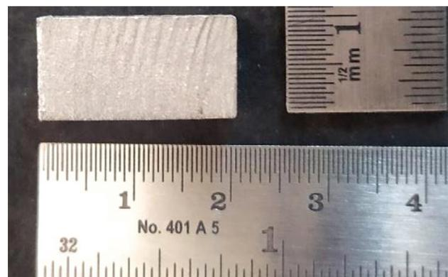
**Figure 3:** Sample machined with AWJM
