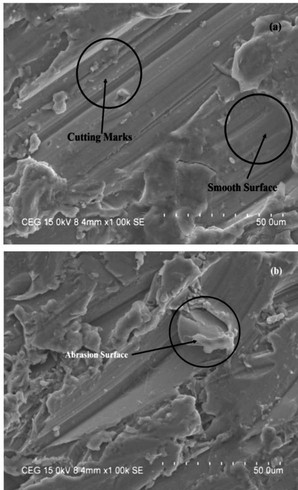
Figure 11: SEM images of the AWJ machined surface: a) mesh size 80 and b) mesh size 120
