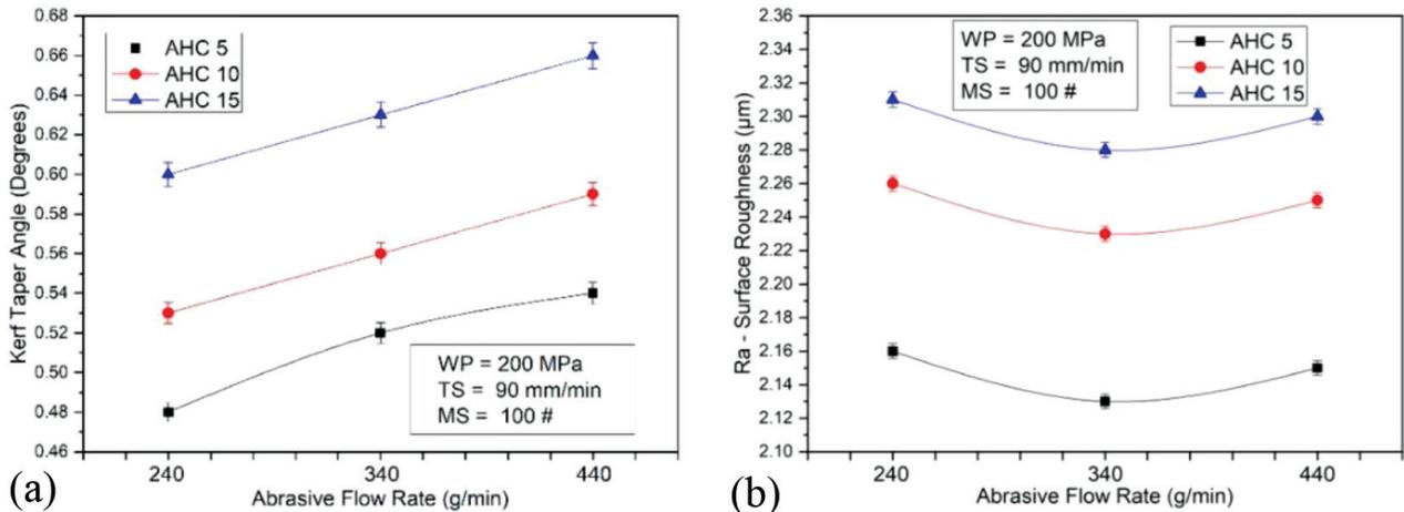
Figure 8: Abrasive flow rate: a) vs kerf taper angle and b) vs surface roughness
