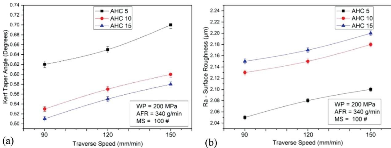
Figure 6: Traverse speed: a) vs kerf taper angle, b) vs surface roughness
