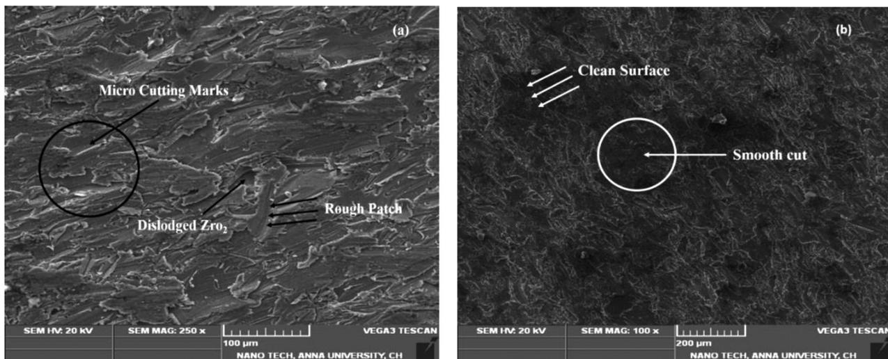
Figure 5: SEM images of AWJ machined surface: a) 125 MPa and b) 275 MPa
