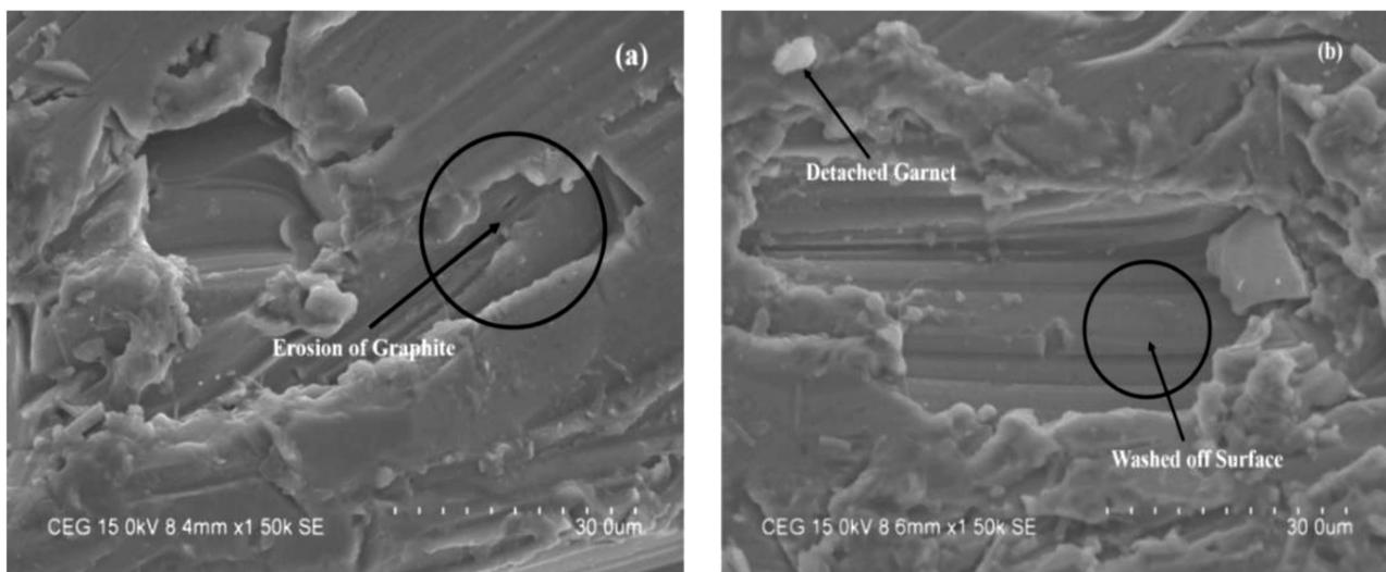
Figure 7: SEM images of the AWJ machined surface: a) 60 mm/min and b) 120 mm/min
