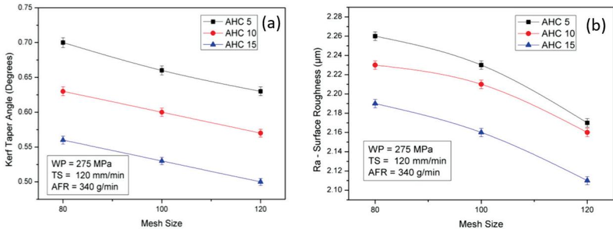
Figure 10: Mesh size: a) vs kerf taper angle and b) vs surface roughness
