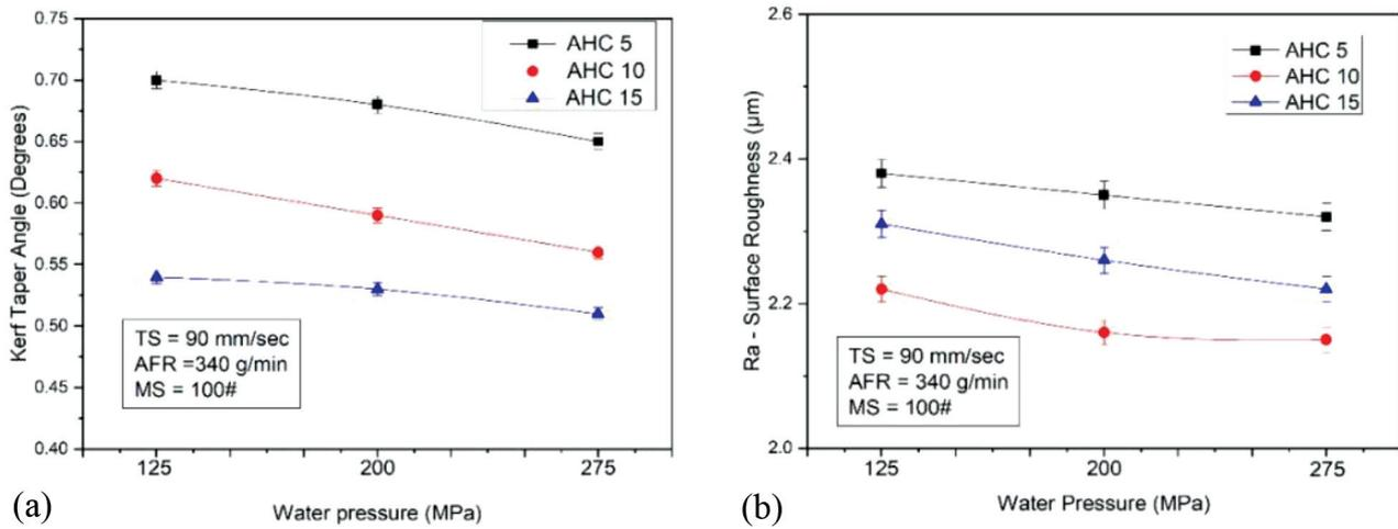
Figure 4: Water pressure: a) vs kerf taper angle and b) vs surface roughness
