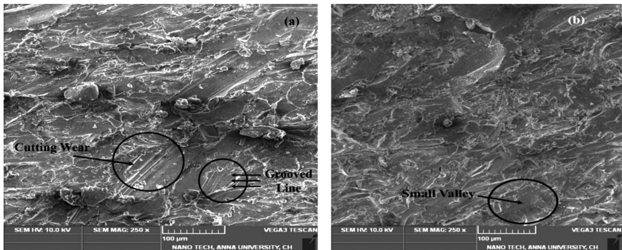
Figure 9: SEM images of the AWJ machined surface: a) 240 g/min and b) 440 g/min
