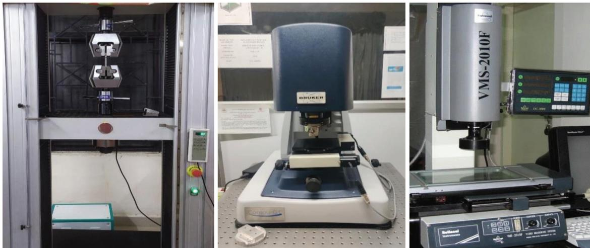
**Figure 2:** Equipment used: a) tensile testing machine, b) surface roughness tester, c) video measuring system
