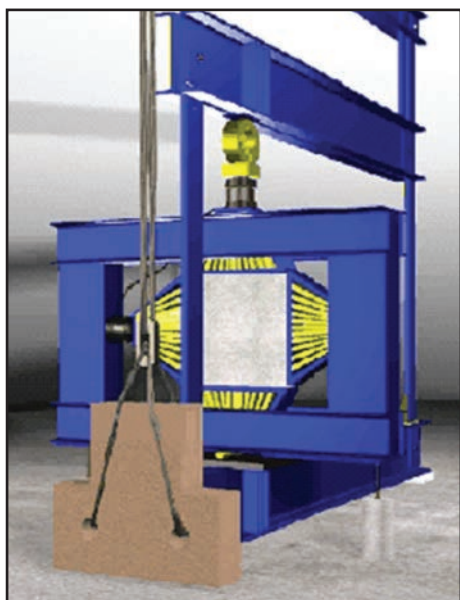
Figure 4. Device for bi-axial loading – characteristic view.
