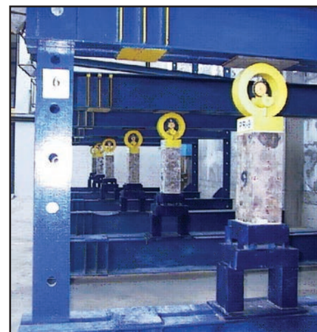
Figure 3. Prismatic sample: a) scheme of measurement points; b) samples during the creep test (coated with paraffin).
