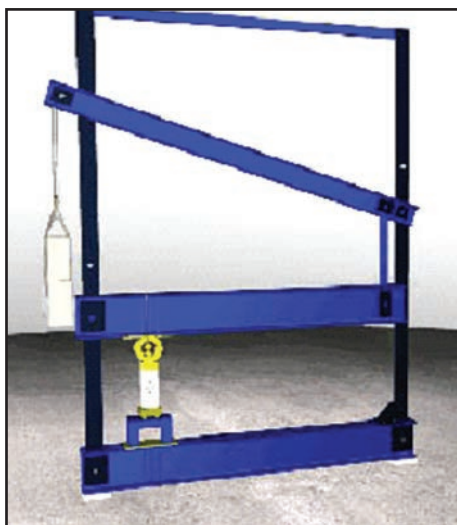
Figure 2. Device for uniaxial loading at creep test.
