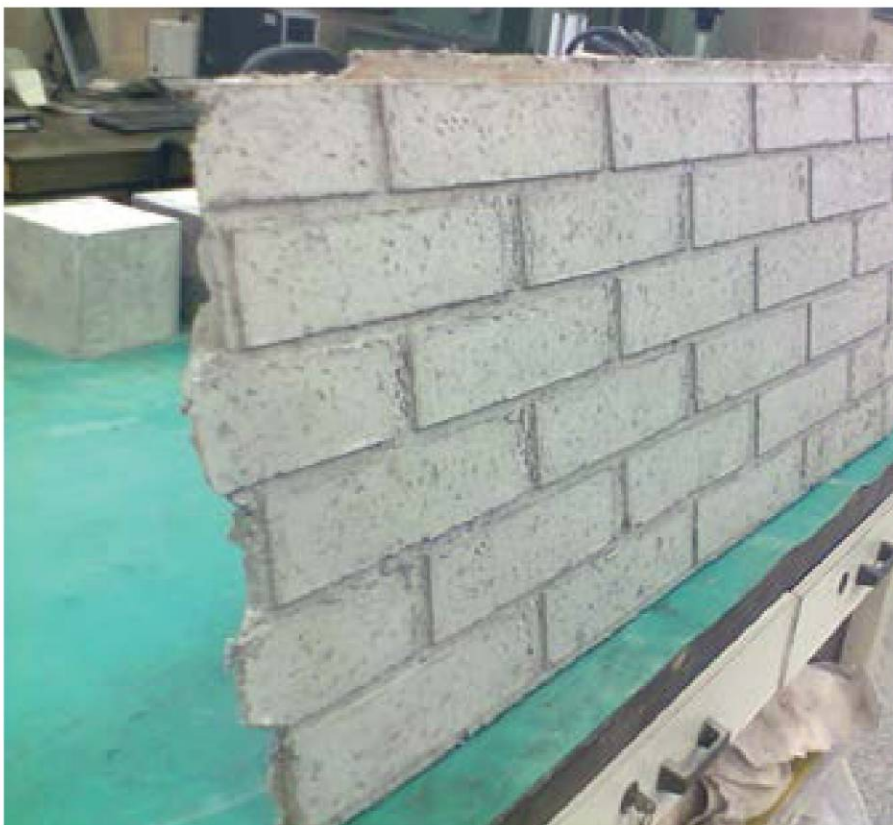
Slika 2: Plošča OPMIS–3 (po razkalupljenju iz »strukturnega« kalupa) Figure 2: Hydraulically bound fibreboard OPMIS–3 (after taken from "structural" mold)
