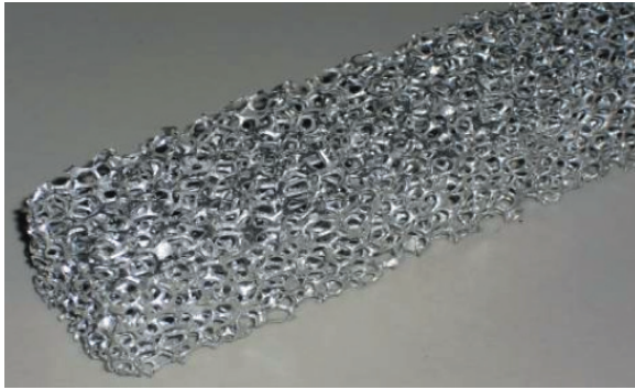
Fig. 5. Insert made of open cell aluminium foam
