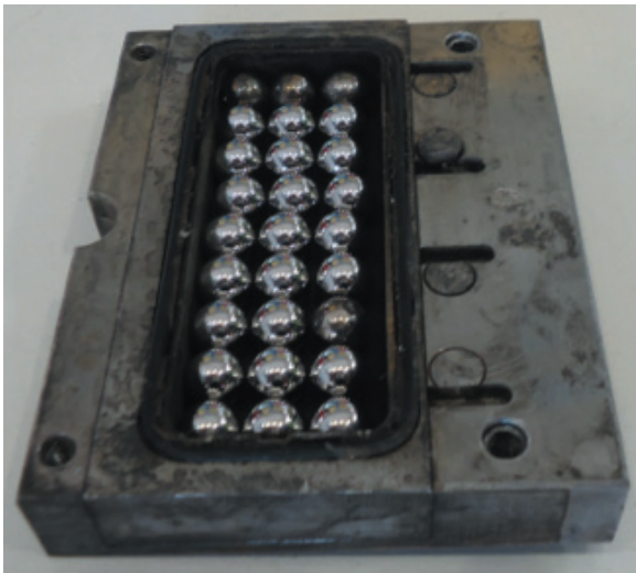
Fig. 6. Mould slot filled with bearing balls
