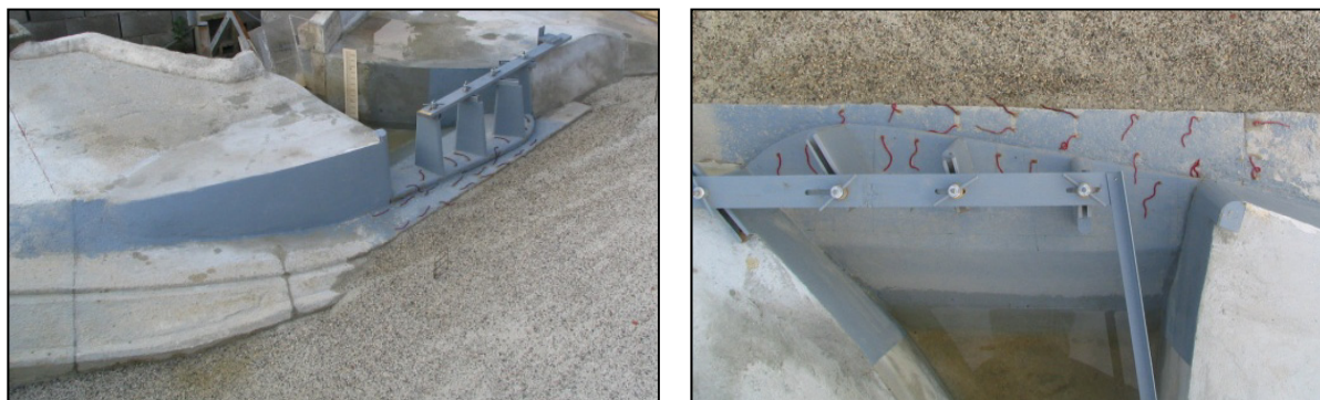
Slika 10: Fizični hidravlični model vtočnega objekta: (a) pogled z desnega brega, (b) tloris Figure 10: Physical hydraulic model of the intake: (a) view from the right bank, (b) plan view
