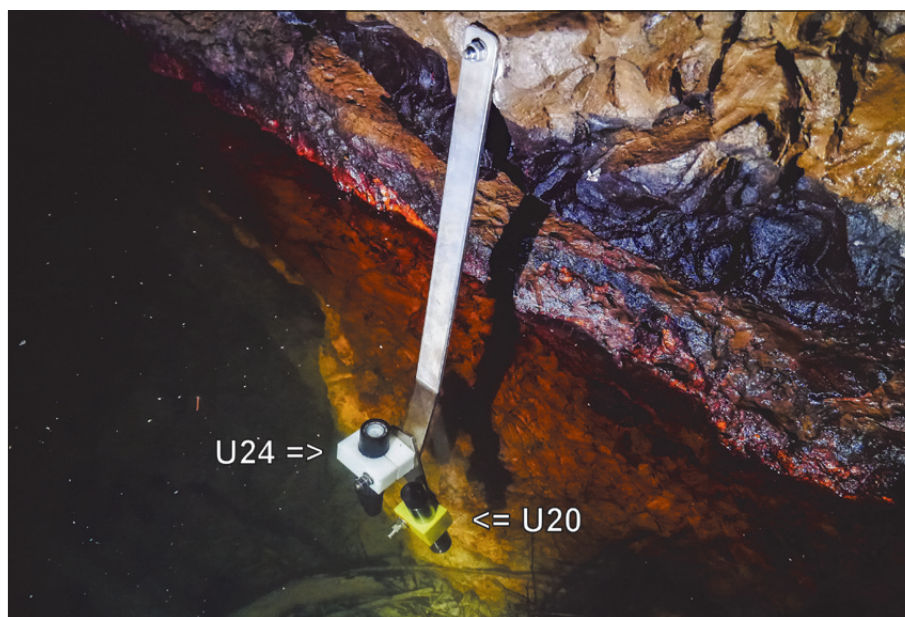
Fig. 3: Typical measurement station with Onset Hobo instruments (left: U24 - temperature and SEC measurements; right: U20 - pressure and temperature measurements). The instruments are installed within a plastic holder attached to the stainless rod, which is fixed to the wall just above the low stand water level (Photo: M. Blatnik)
