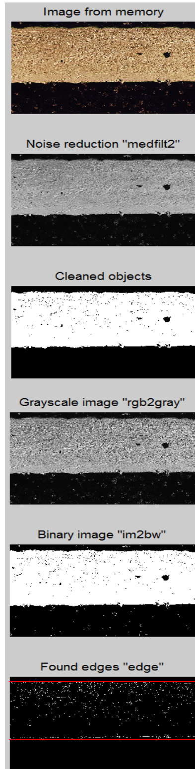
Fig. 11 Algorithm testing for second metallographic microscopic image, d = 920.4 \mu\text{m}
