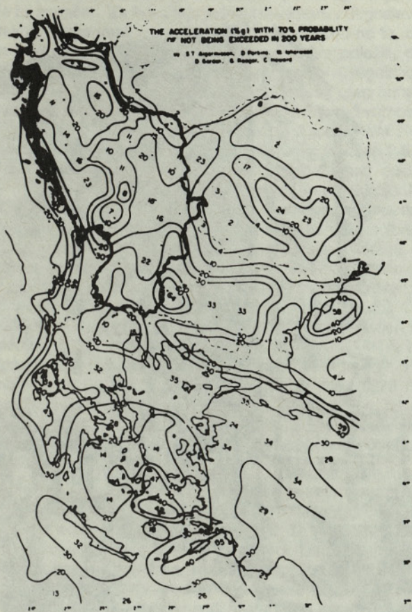
Figure 10 - Acceleration with 70 percent probability of not being exceeded in 200 years
