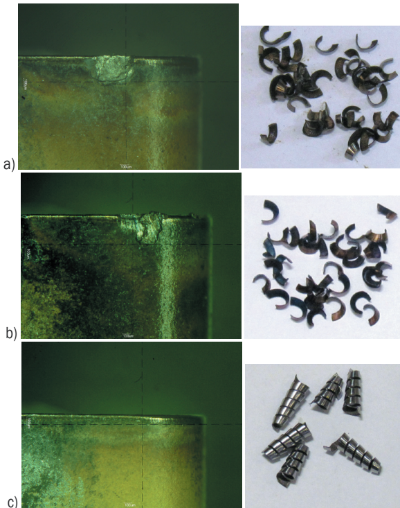
Fig. 6. Flank tool wear and chip shape ( a_p = 2 mm, f = 0.28 mm·rev -1 , v_c = 320 m·min -1 ) for: a) conventional, b) MQL and c) HPJAM
