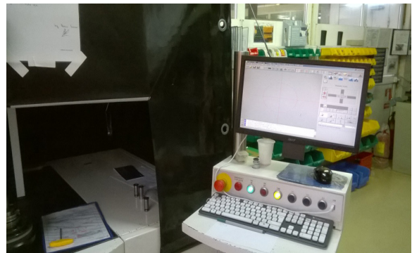
Fig. 5. Walter Helicheck Basic, optical CNC measuring machine
