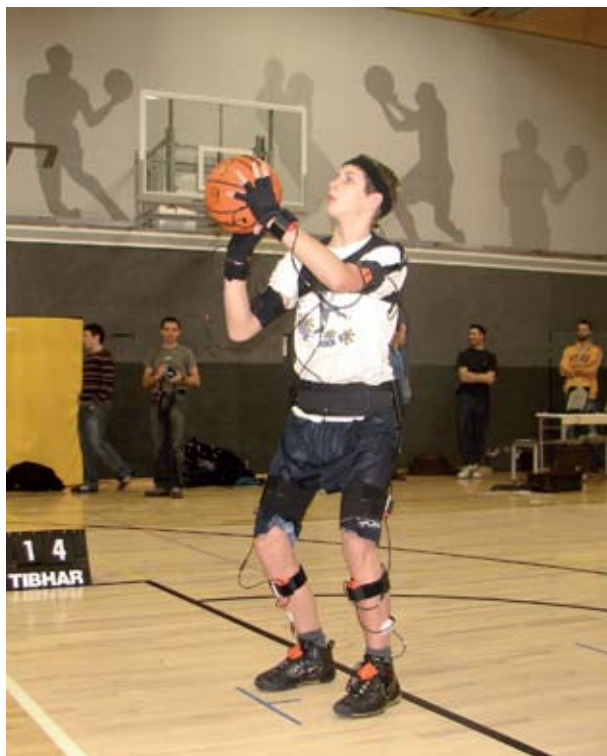
Figure 2. The kinematic parameters during a jump shot were measured using the inertial suit “MVN”
