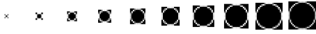
Figure 4. Filters \mathcal{A}_m(x, y); m = 1, \dots, M - 1 . The radial detector uses 11 circles to compute the saliency maps. The sum of the pixel weights is for each circle equal to N . The first filter \mathcal{A}_0(x, y) with r_m = 0 , not shown in the image, just multiplies the image intensity with N .
