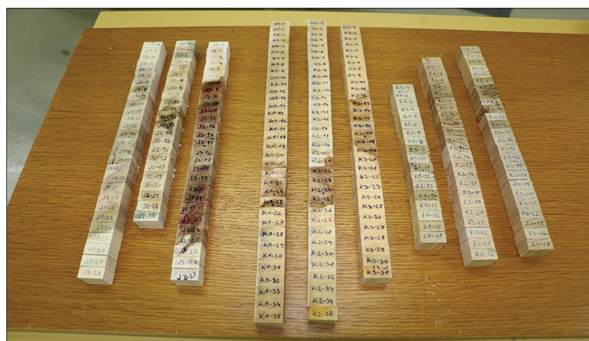
Figure 1. Samples cut from the central board to determine the radial density and moisture content profile (from periphery through pith to periphery of the stem) of box elder, horse chestnut and black locust.
