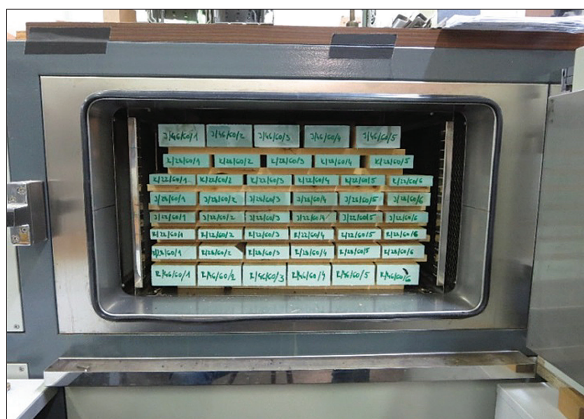
Figure 2. Experimental drying chamber with wood samples.
