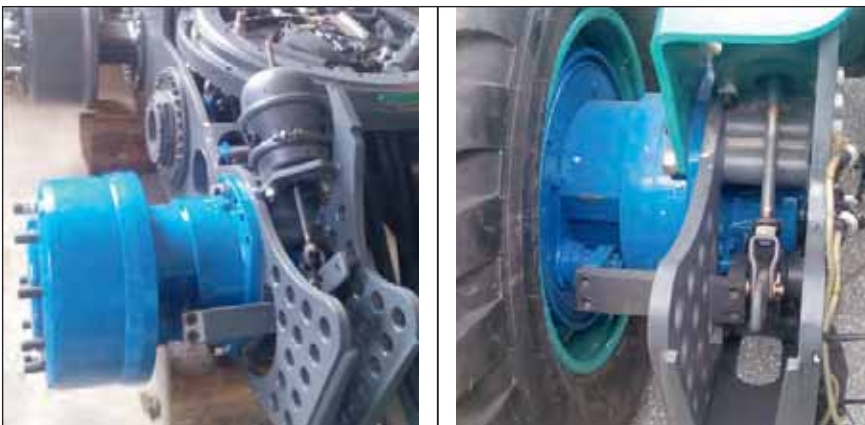
Figure 4. Wheel type hydraulic motors
