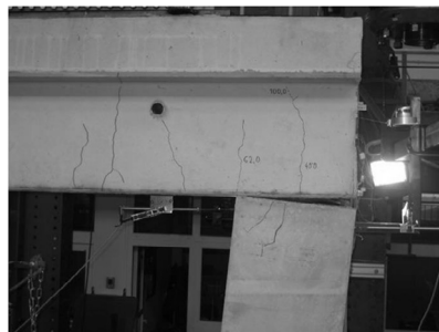
Fig. 11. Large relative rotations between the beam and the column.
