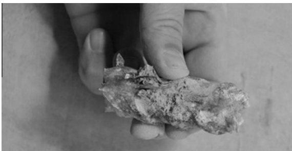
Fig. 9. At the end of the cyclic test the dowel was broken at two levels. The distance between the two locations was about 8 cm.
