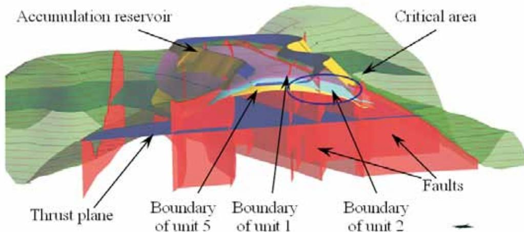
Figure 7. Critical cross-section of the reservoir model.
