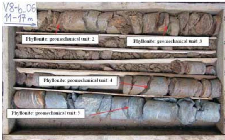
Figure 4. Typical geomechanical units of phyllonite shown in the borehole core.
