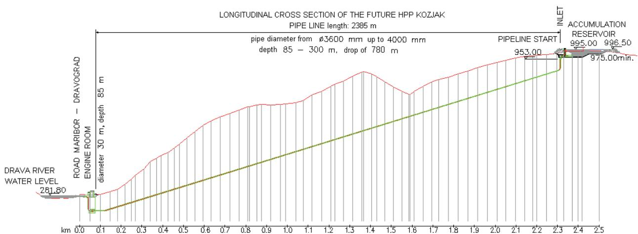
Figure 2. Longitudinal cross-section of Kozjak HPP.
