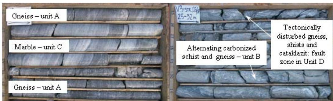
Figure 8. Most common lithological units in the area of the engine room.
