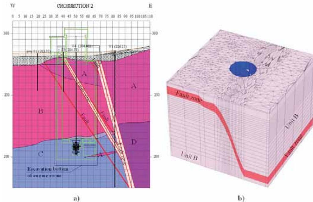
Figure 11. a) Most critical cross-section in the engine-room area, b) 3D numerical model.
