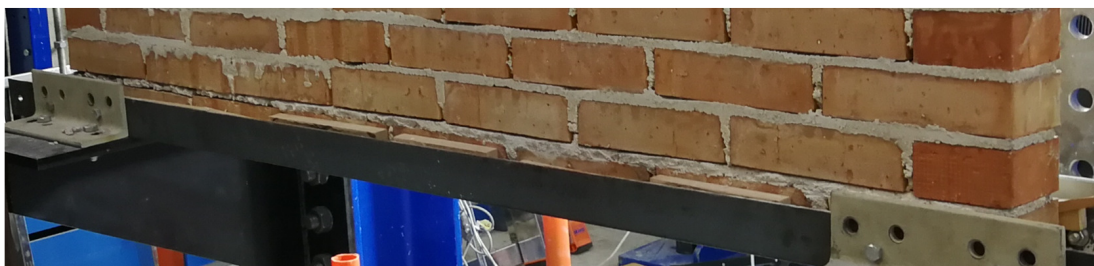
Slika 7.4: Nepopolno zapolnjena horizontalna spojnica med 1. in 2. vrsto zidakov pri preizkušancu NF-3. Figure 7.4: Imperfectly filled horizontal bed-joint between the first and second row of bricks of the NF-3 specimen.
