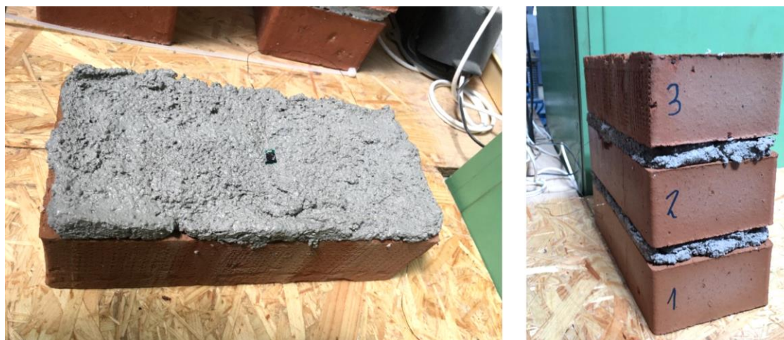
Slika 4.28: Prikaz vgradnje senzorjev UL FE v spojnico (levo) preizkušanca in cel preizkušaneč (desno). Figure 4.28: Installation of UL FE sensor in a bed joint of a masonry specimen (left) and a finished specimen (right).
