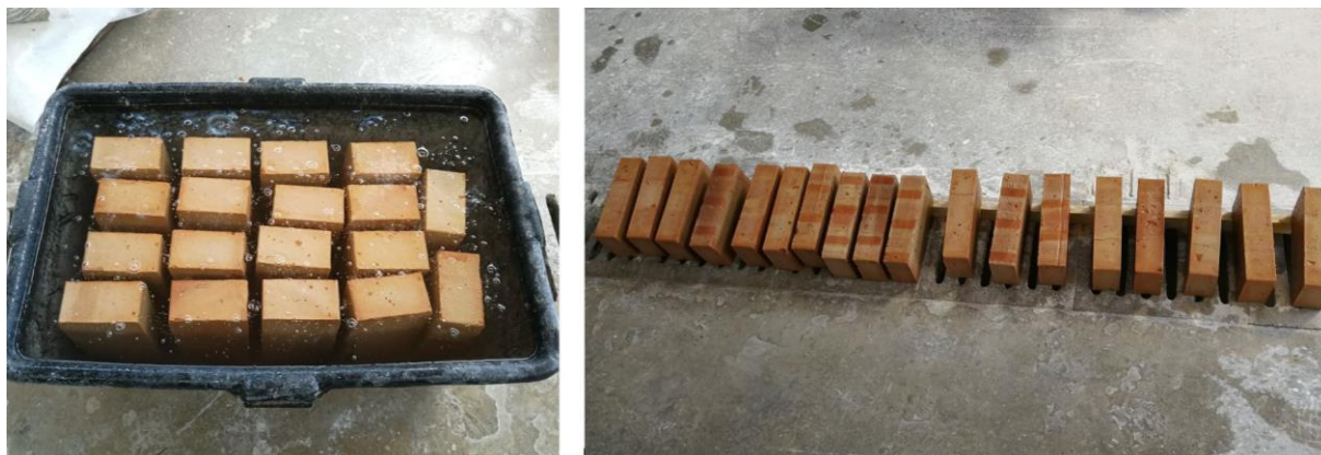
Slika 4.2: Namakanje zidakov NF (levo) in odcejanje zidakov NF (desno). Figure 4.2: Submerged NF bricks (left) and NF bricks during draining (right).
