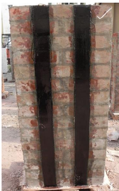
Slika 2.10: CFRP utrditveni sistem (Padalu et al., 2019). Figure 2.10: CFRP strengthening system (Padalu et al., 2019).
