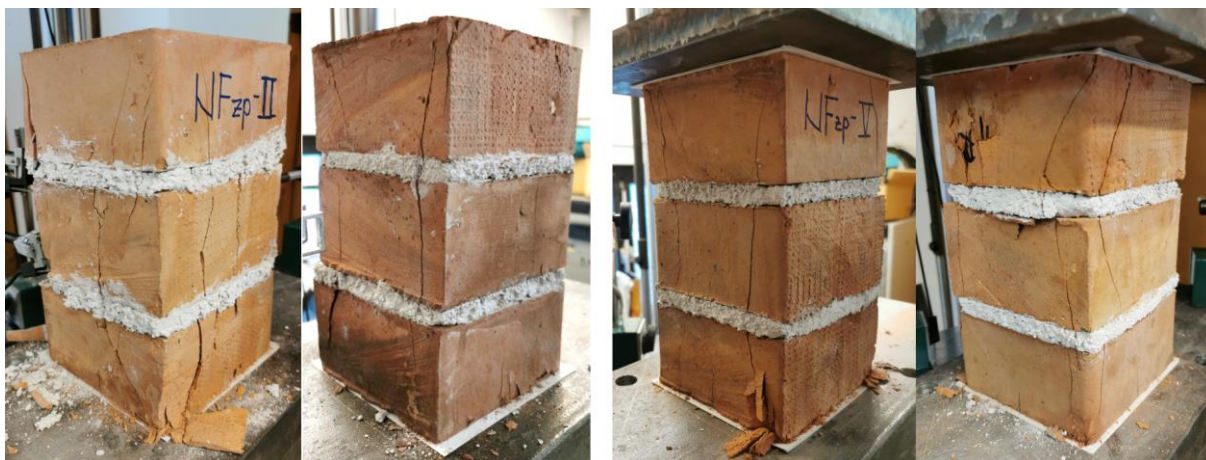
Slika 4.23: Primera porušitve vzorcev zidanih prizem po tlačni preiskavi. Figure 4.23: Two examples of masonry prisms' failure after compression test.
