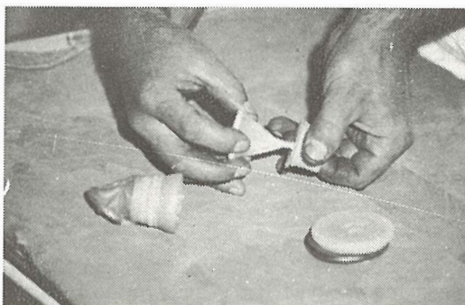
Fig. 2 – Torsion of the elastic tube – emphasis on the small bulge of the rubber tube, which connects both pieces
